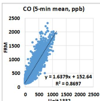
Coefficient of Determination ( $R^2$ ) quantifies how the three sensors followed the CO concentration change by FRM.
