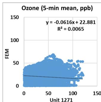
Coefficient of Determination ( $R^2$ ) quantifies how the three sensors followed the O<sub>3</sub> concentration change by FEM.
