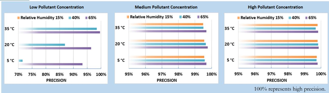
Sensor's ability of generating precise measurements of O<sub>3</sub> concentration at low, medium, and high pollutant levels were evaluated under 9 combinations of T and RH, including extreme weather conditions like cold and humid (5 °C and 65%), hot and humid (35 °C and 65%), cold and dry (5 °C and 15%), and hot and dry (35 °C and 15%).
