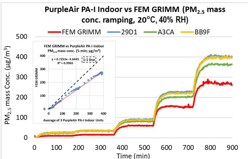
The PA-I Indoor sensors showed very strong correlations with the corresponding FEM PM<sub>2.5</sub> data ( $R^2 > 0.99$ ) at 20 °C and 40% RH. For conc. ramping experiments of PM<sub>1.0</sub> and PM<sub>10</sub>, please see the lab report.
