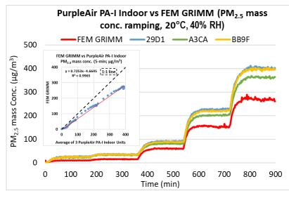
The PA-I Indoor sensors showed very strong correlations with the corresponding FEM  $PM_{2.5}$  data ( $R^2 > 0.99$ ) at 20 °C and 40% RH. For conc. ramping experiments of  $PM_{1.0}$  and  $PM_{10}$ , please see the lab report.
