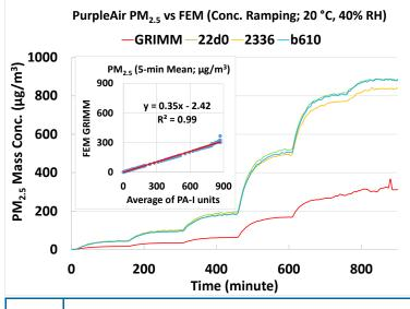
The three PA-I sensors showed very strong correlations with the corresponding FEM  $PM_{2.5}$  data ( $R^2 = 0.99$ ) at 20 °C and 40% RH.
