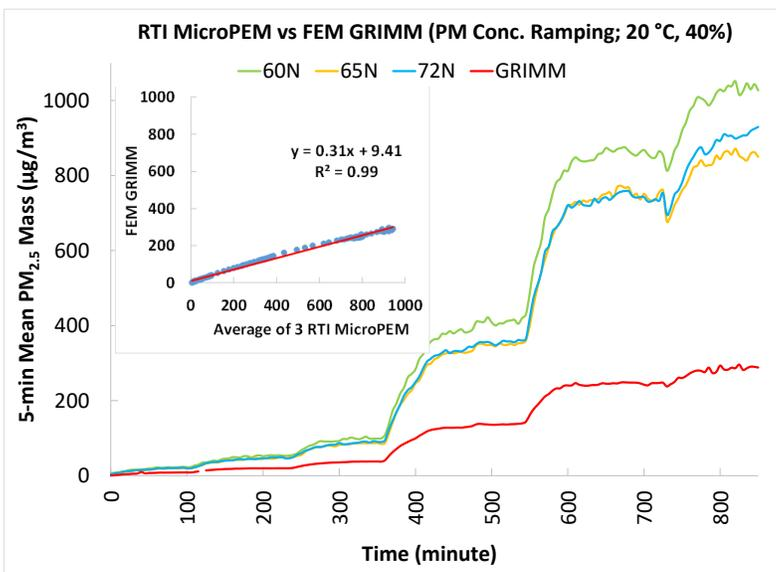
The three RTI MicroPEM sensors showed very strong correlations with the corresponding FEM PM<sub>2.5</sub> data ( $R^2 = 0.99$ ) at 20 °C and 40% RH from 0 - 250 µg/m<sup>3</sup>.
