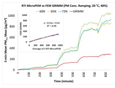
The three RTI MicroPEM sensors showed very strong correlations with the corresponding FEM PM<sub>2.5</sub> data ( $R^2 = 0.99$ ) at 20 °C and 40% RH from 0 - 250  $\mu$ g/m<sup>3</sup>.
