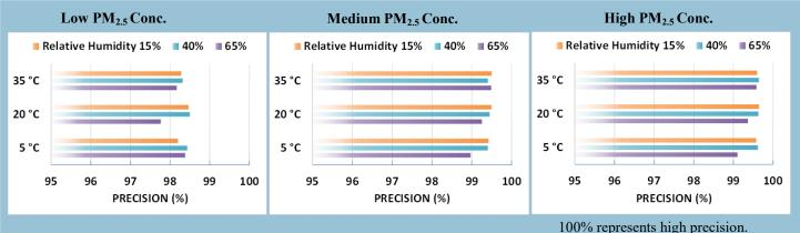
Sensor ability of generating precise measurements of PM concentration at low, medium, and high pollutant levels were evaluated under 9 combinations of T and RH, including extreme weather conditions like cold and dry (5 °C and 15%), cold and humid (5 °C and 65%), hot and humid (35 °C and 65%), or hot and dry (35 °C and 15%).
