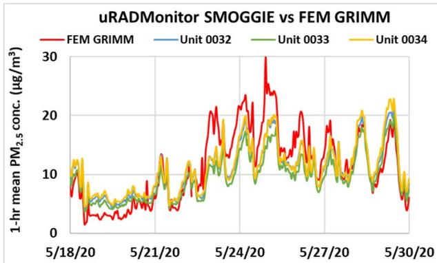
Coefficient of Determination ( $R^2$ ) quantifies how the three sensors followed the PM<sub>2.5</sub> concentration change by the reference instruments.
