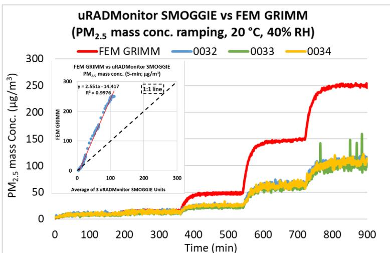
The uRADMonitor SMOGGIE sensors showed very strong correlations with the corresponding FEM PM<sub>2.5</sub> data ( $R^2 > 0.99$ ) at 20 °C/40% RH.. For conc. ramping experiments of PM<sub>1.0</sub>, please see the lab report.
