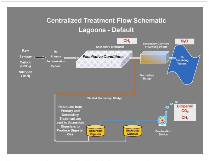
The methane emissions expected from facultative lagoons are calculated using Equation 10.3 from LGOP:
