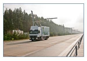
Figure 5Truck Catenary (Siemens)
