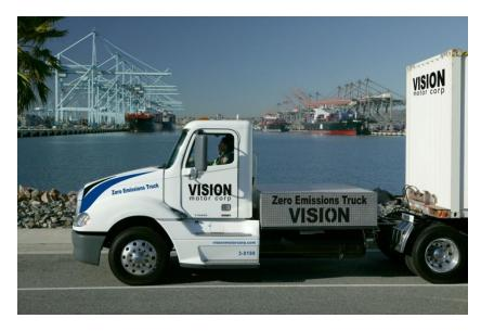
Figure 2 Vision Zero-Emission Fuel Cell Battery Electric Truck
