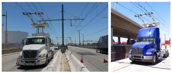
TransPower Catenary Truck on the OCS Track
