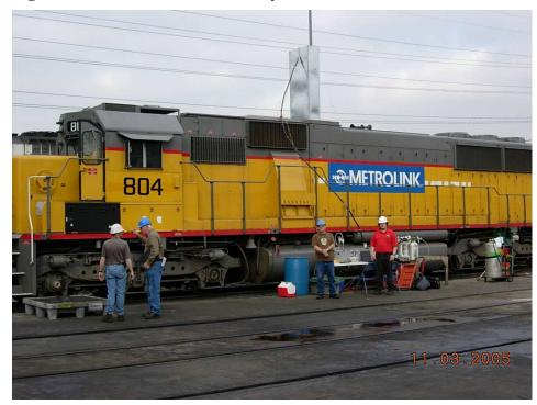
Figure 1: Emission measurement system installation on Metrolink No. 804
