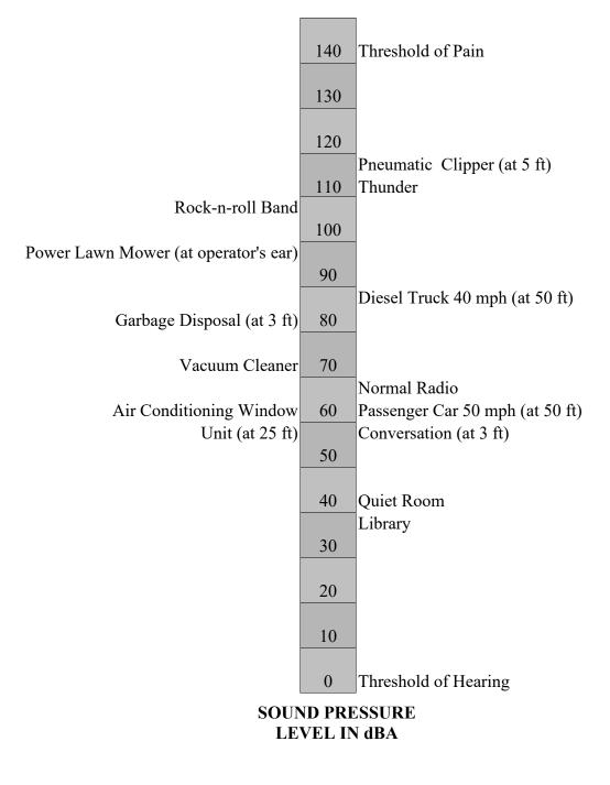
FIGURE 3.6-1 General Noise Sources and Associated Sound Pressure Levels
