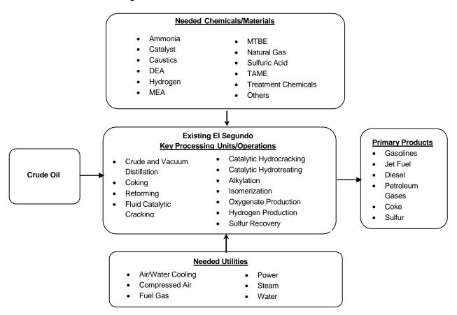
Figure 2.5-1 Simplified Block Diagram – Chevron El Segundo Refinery
