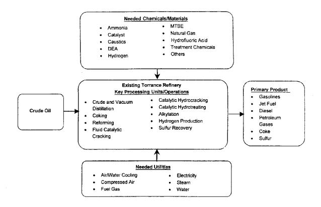
Figure 2.3-1 Simplified Block Diagram – Mobil Torrance Refinery
