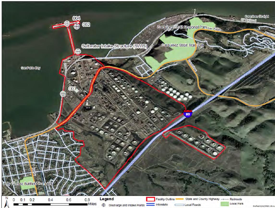
**Map 1. Rodeo facility outline, discharge points, and intake points.** Attachment B to NPDES Permit, Order R2-2011-0027. The left-most circle containing a cross denotes discharge point E-003.
