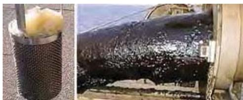
**Fig. 4.** Waxy deposits removed from shale oil pipelines.
