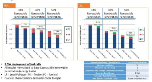
Figure 1: Grid Simulation Modeling of 5 GW Fuel Cell Deployment in California with Different Renewable Penetrations<sup>2</sup>
