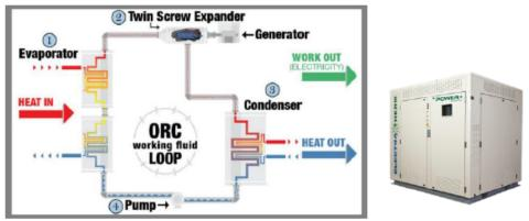
No gearbox, combustion, air filters, or exhaust stack. Low temperature (170F-252F) hot water is the fuel.
