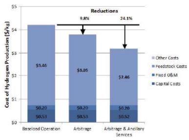
Figure 7 – Potential Incremental Value of Electrolyzer Providing Grid Services
