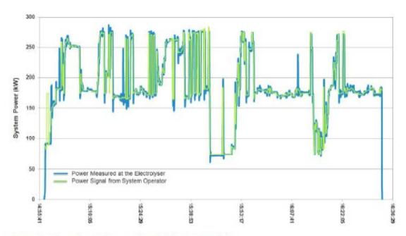
Figure 2 - Electrolyzer Sub-second Load Following Capability
