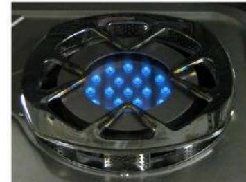
US application #15/942,915 filed on April 2, 2018, "Apparatus and Method for Burning a Lean, Premixed flame"
