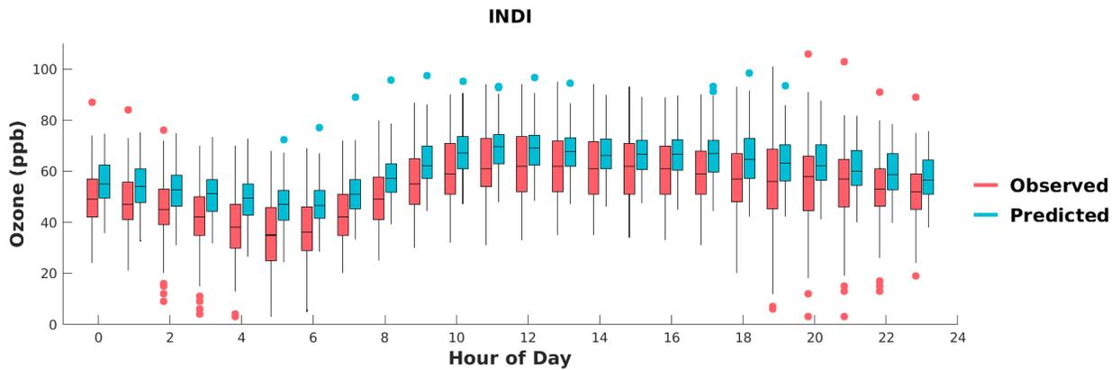
**FIGURE F-12: BOX PLOTS OF OBSERVED VS. PREDICTED HOURLY OZONE DURING MAY 1<sup>ST</sup> TO SEPTEMBER 30<sup>TH</sup>, 2018, AT INDIO. HORIZONTAL LINES INDICATE 25<sup>TH</sup>, 50<sup>TH</sup> (MEDIAN), AND 75<sup>TH</sup> PERCENTILES.**
