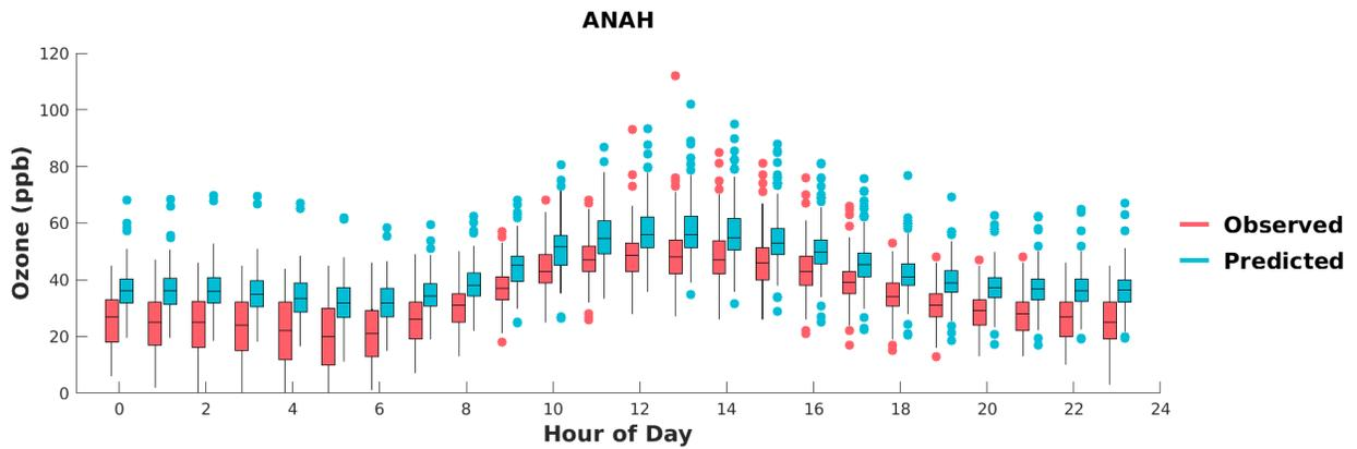
**FIGURE F-1: BOX PLOTS OF OBSERVED VS. PREDICTED HOURLY OZONE DURING MAY 1<sup>ST</sup> TO SEPTEMBER 30<sup>TH</sup>, 2018, AT ANAHEIM. HORIZONTAL LINES INDICATE 25<sup>TH</sup>, 50<sup>TH</sup> (MEDIAN), AND 75<sup>TH</sup> PERCENTILES.**
