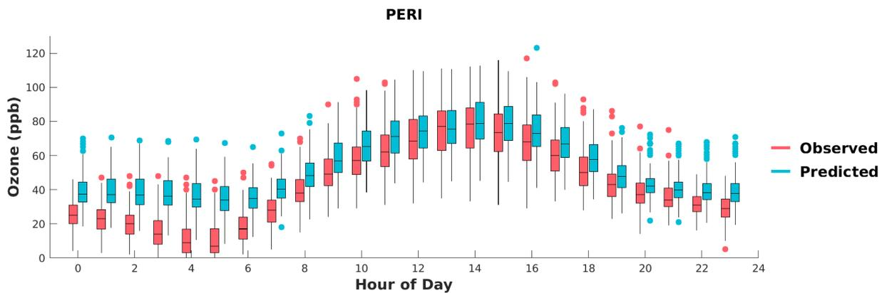
**FIGURE F-18: BOX PLOTS OF OBSERVED VS. PREDICTED HOURLY OZONE DURING MAY 1<sup>ST</sup> TO SEPTEMBER 30<sup>TH</sup>, 2018, AT PERRIS. HORIZONTAL LINES INDICATE 25<sup>TH</sup>, 50<sup>TH</sup> (MEDIAN), AND 75<sup>TH</sup> PERCENTILES.**
