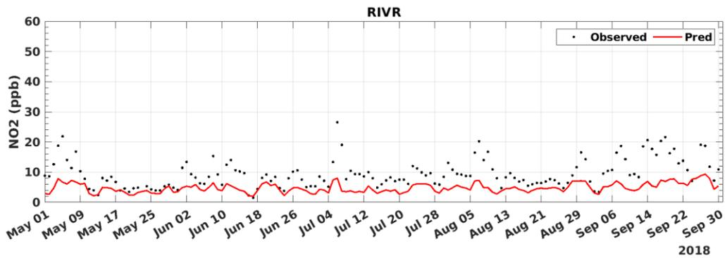
FIGURE C-17: 2018 DAILY AVERAGED NO2 MODEL PREDICTION AND MEASUREMENT COMPARISON AT RIVERSIDE
