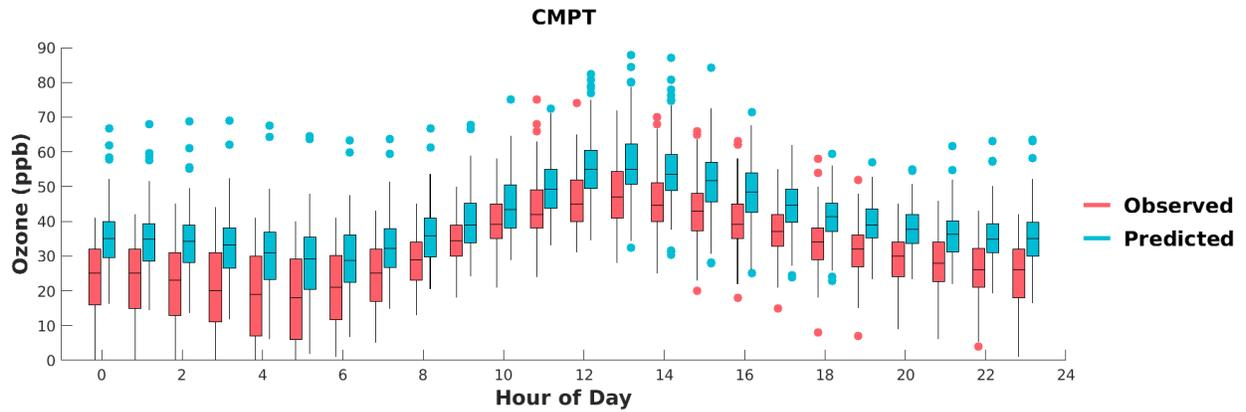
**FIGURE F-5: BOX PLOTS OF OBSERVED VS. PREDICTED HOURLY OZONE DURING MAY 1<sup>ST</sup> TO SEPTEMBER 30<sup>TH</sup>, 2018, AT COMPTON. HORIZONTAL LINES INDICATE 25<sup>TH</sup>, 50<sup>TH</sup> (MEDIAN), AND 75<sup>TH</sup> PERCENTILES.**
