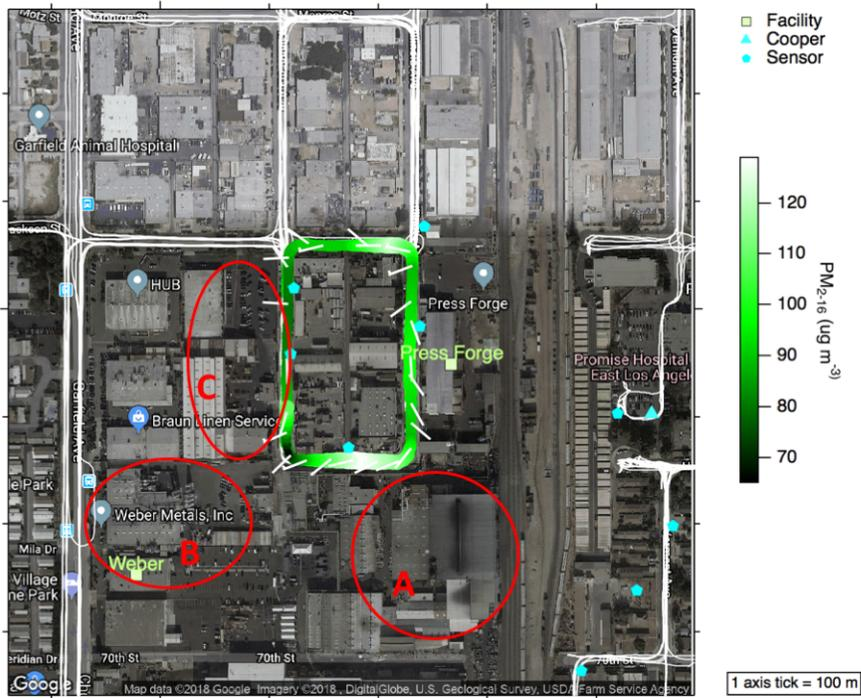
Figure 13. Map of apparent emission zones to the West of Promise Hospital, Paramount. The white lines represent the total project GPS track of the AML. The shaded data points (black-green-white color scale) are PM response for a period on April 5<sup>th</sup>, 2018. The red circled areas are potential source regions.
