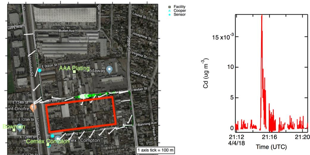
Figure 41. Example Cd plume in North Compton. The suspected source location is inside the city block outlined in red. No specific business could be conclusively identified as a Cd source.
