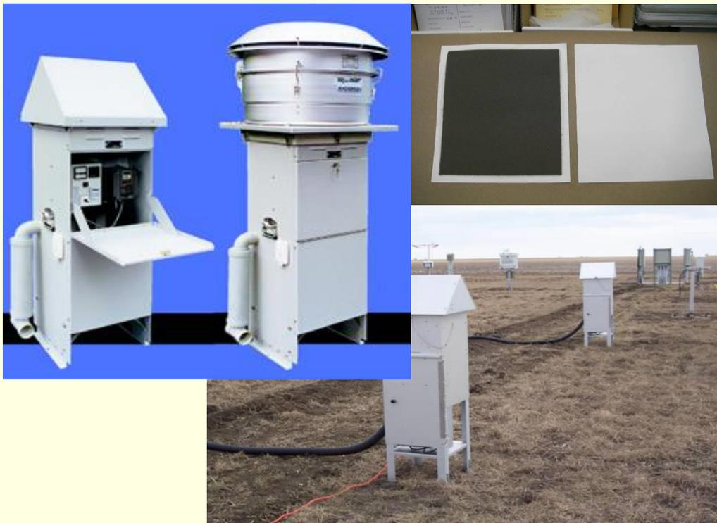
Levels are determined weighing by the difference between upwind & downwind samples trapped in the high volume particulate filters over a 5 hour period
