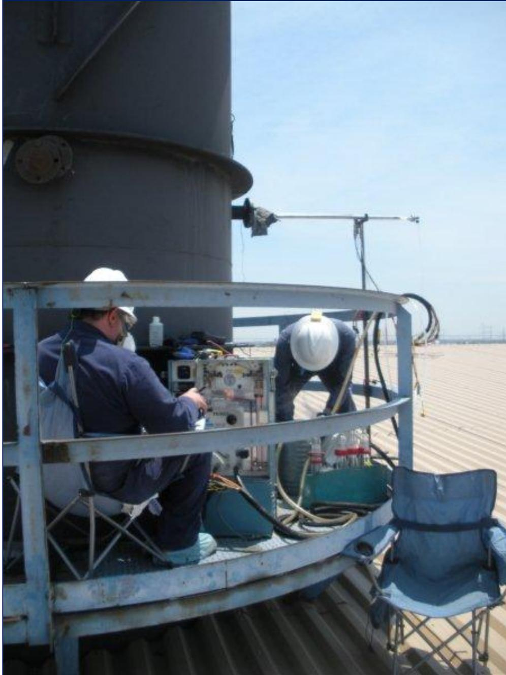
**Figure 6: CARB Method 436 Field Sampling Train and Probe**
