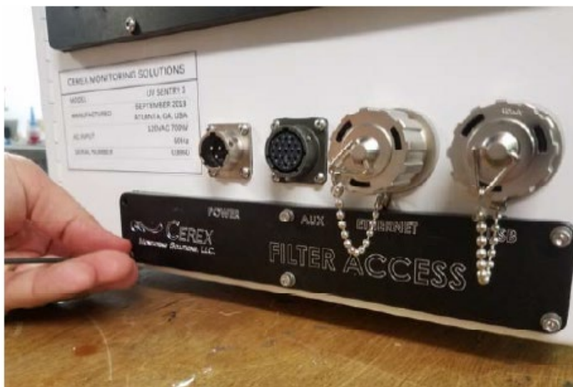
Figure 5. Location of filter access plate.
