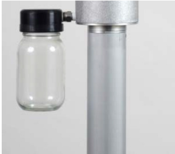
Figure 23. Water collector attached to inlet.
