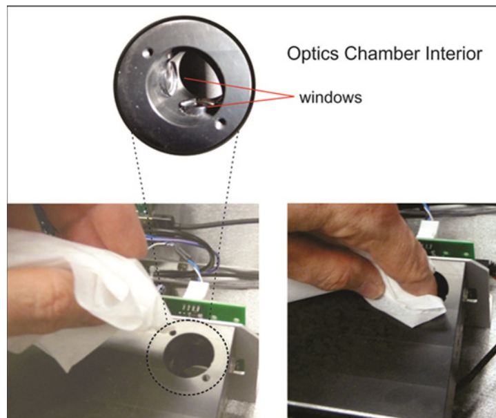
Figure 10. Maintenance: optics chamber windows.
