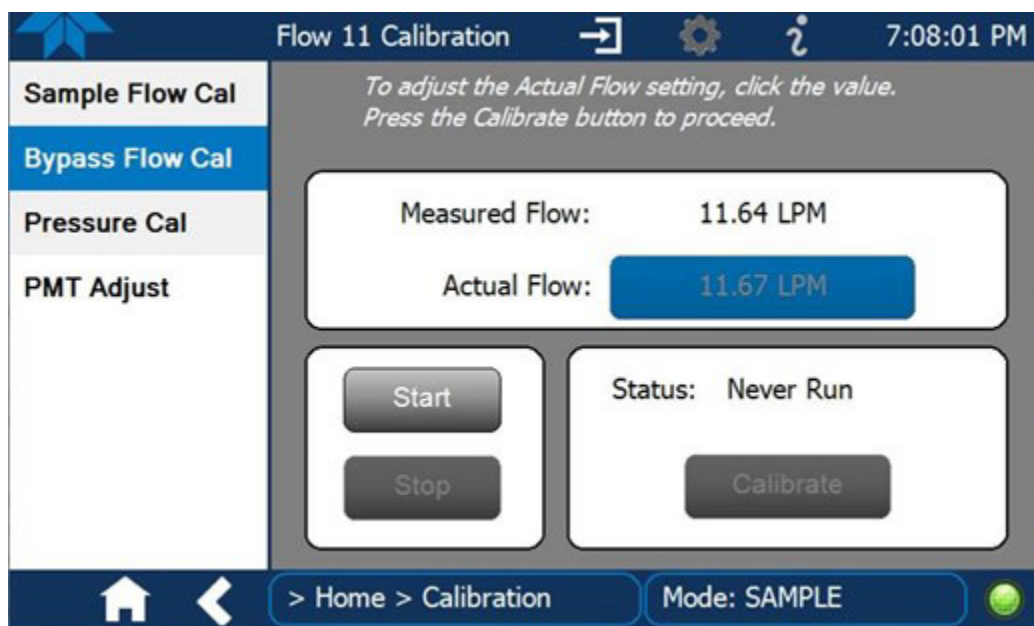
Figure 19. Bypass Flow calibration screen.
