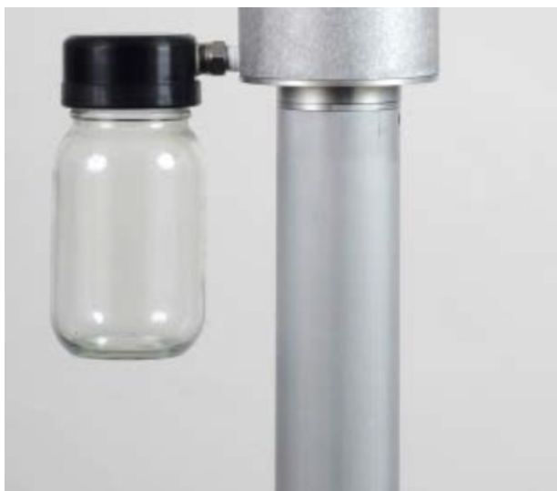
Figure 23. Water collector attached to inlet.
