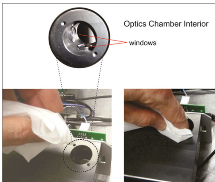
Figure 10. Maintenance: optics chamber windows.
