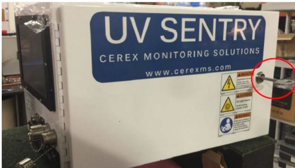
Figure 9. Opening the source access panel.
