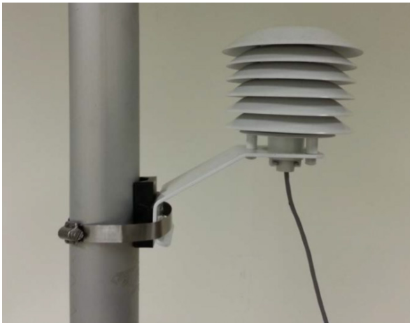
Figure 26. Ambient temperature probe installed in the solar shield.
