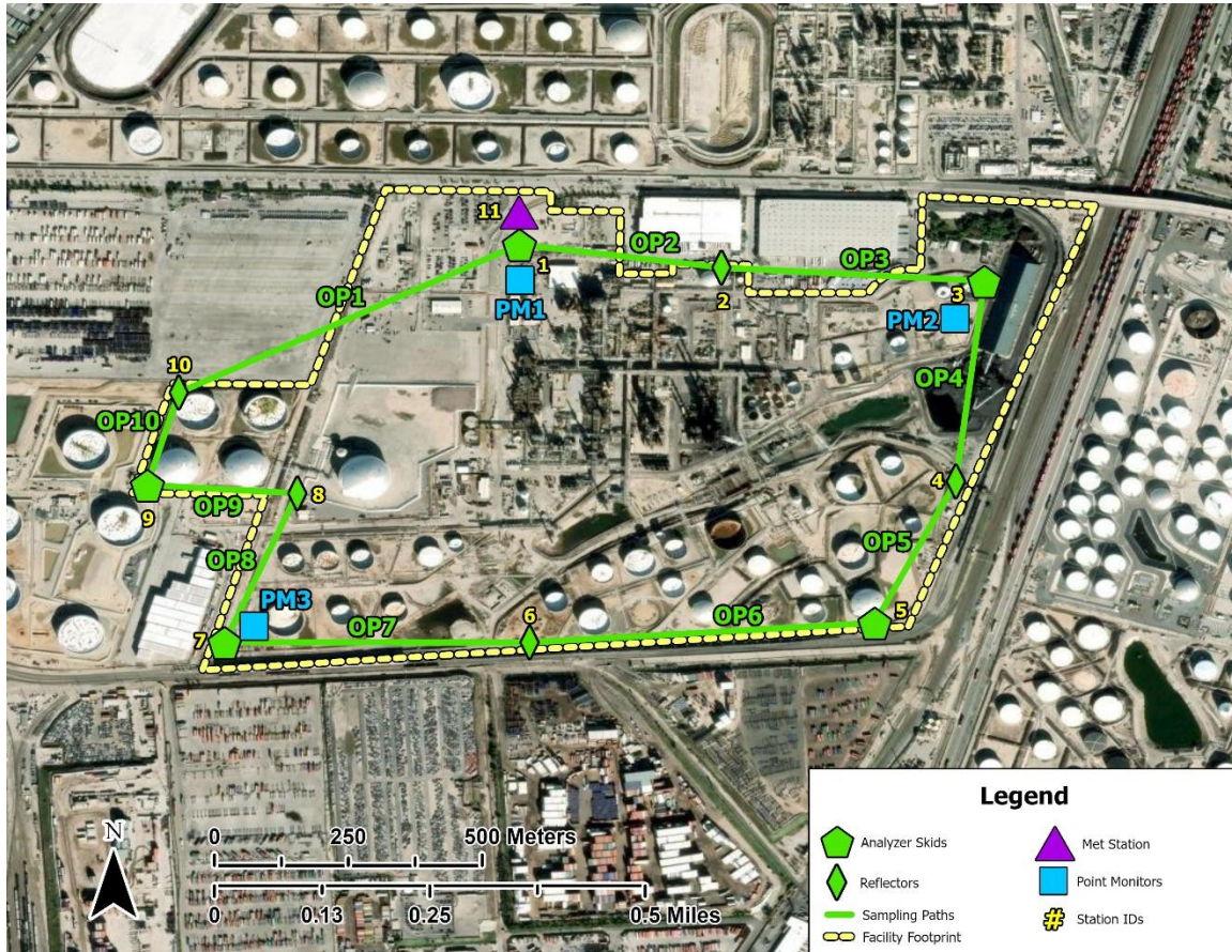
Figure 1. Fenceline monitoring sampling locations for the P66 Carson Refinery.
