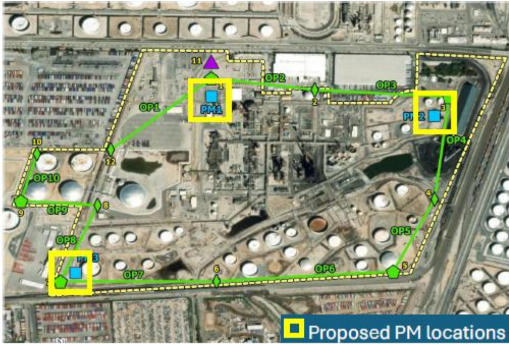
Figure 29. Fenceline monitoring sampling locations for implementation prior to restart of refinery operations from idling for the P66 Carson Refinery. Yellow squares indicate proposed point monitor (PM) locations as proposed by South Coast AQMD.
