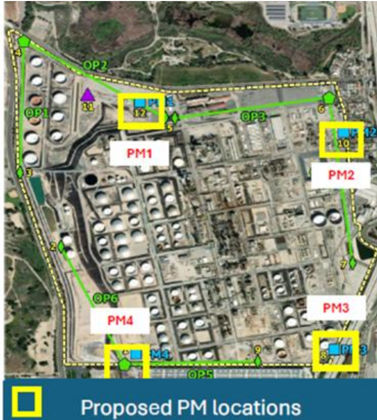
Figure 31. Fenceline monitoring sampling locations for implementation prior to restart of refinery operations from idling for the P66 Wilmington Refinery. Yellow squares indicate proposed point monitor (PM) locations as proposed by South Coast AQMD.
