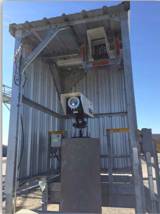
Figure 17. An example of a UVDOAS analyzer (may not be configuration of actual installation).
