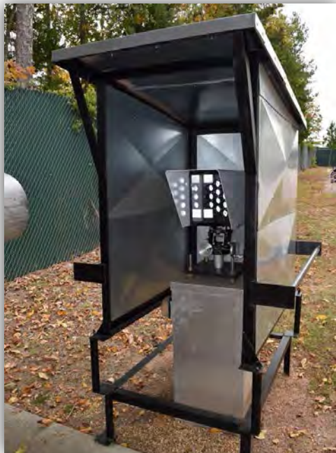
Figure 18. An example of a UVDOAS retroreflector (may not be configuration of actual installation).
