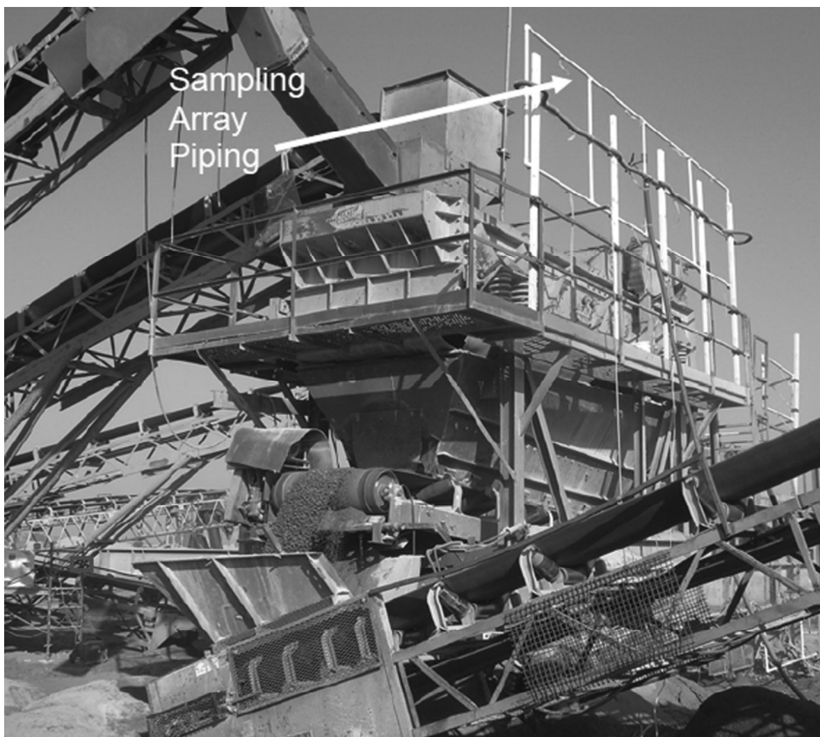
Figure 1. Side view of the sampling array on the downwind side of the vibrating sizing screen at the Barstow plant.
