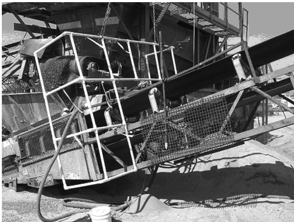
Figure 3. Close-up view of the sampling orifices in the conveyor transfer point array at the Carroll Canyon plant.
