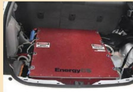
pioneered the engineering and development of the plug-in hybrid-electric vehicle Toyota Prius retrofit. This modified vehicle is designed to achieve more than 100 mpg for the first 50 to 60 miles of a user's daily commute.
