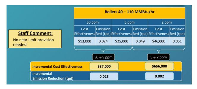
The boilers 40 to 110 MMBtu/hr consist of three boilers located at one facility. These boilers currently do not have NOx controls, so no conditional limit is necessary for this category. Cost-effectiveness was calculated based on cost provided by the facility and is below \$50,000 per ton of NOx. Staff's proposed BARCT limit for the category is 5 ppmv.
