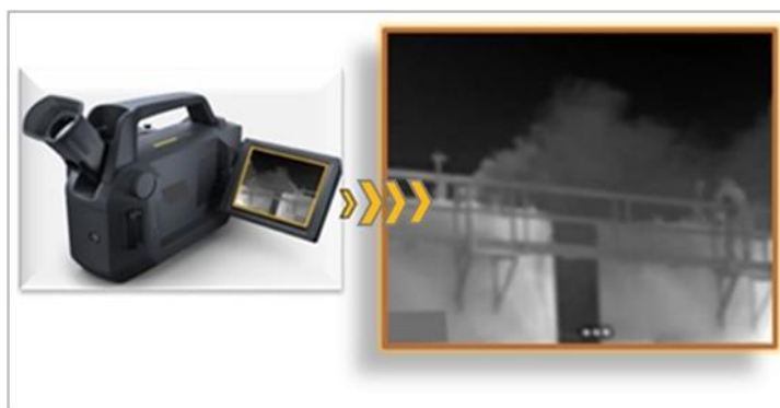
Figure 2.4 – OGI Camera Imaging
