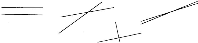
Count as 3 structures if space between fibers is greater than width of 1 fiber diameter or if the number of intersections is equal to or less than 2.
