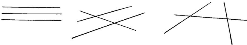
Count bundles as 1 structure; 3 or more parallel fibrils less than 1 fiber diameter separation.
