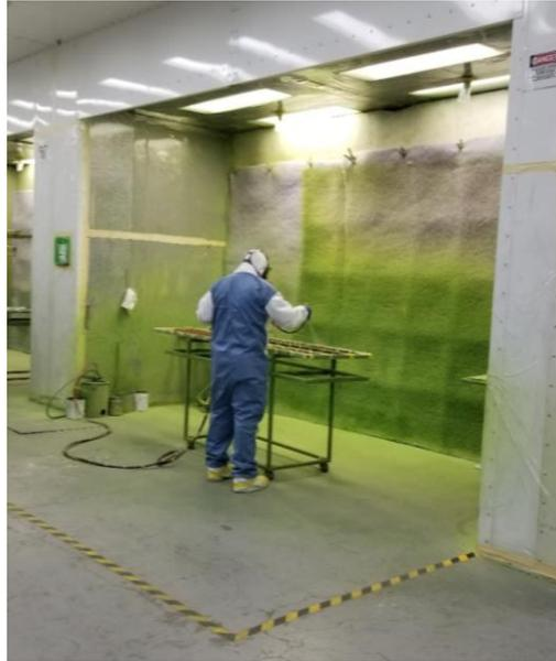
**Figure 2 – Examples of Enclosed Non-Bench Spray Booths**
