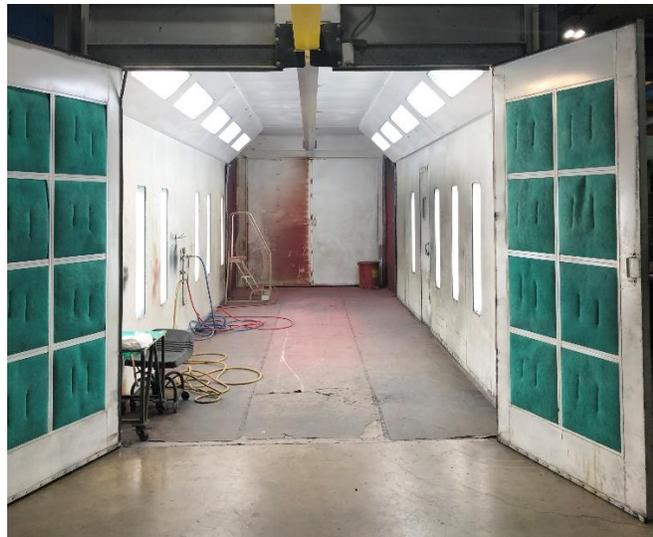
**Figure 3 – Example of an Open Face Bench Spray Booth<sup>5</sup>**
