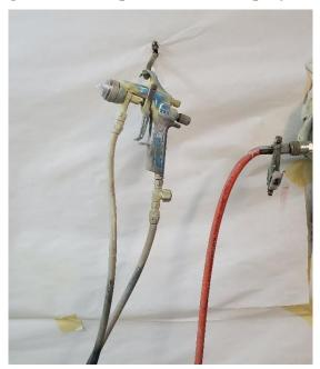
Figure 5 – Example of an HVLP Spray Gun
