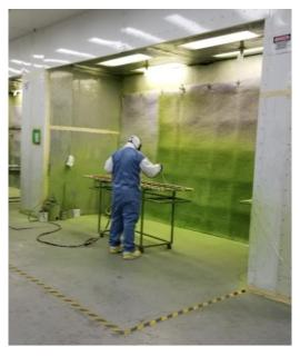
Figure 1 – Example of an Open Face Non-Bench Spray Booth
