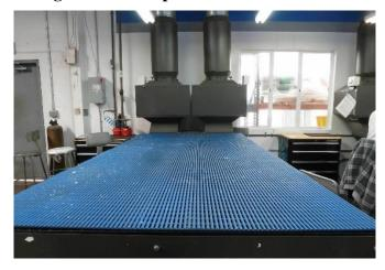
Figure 6 – Example of a Downdraft Table
