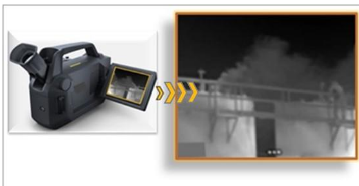
Figure 2.4 – OGI Camera Imaging
