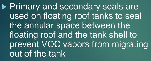
Rule 463 does not require both a primary seal and secondary seal on all floating roof tanks
