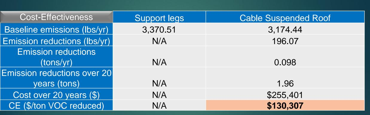
Retrofitting IFR tanks with cable suspended roofs is not cost-effective, therefore staff is not considering requiring the use of cable suspended roofs
