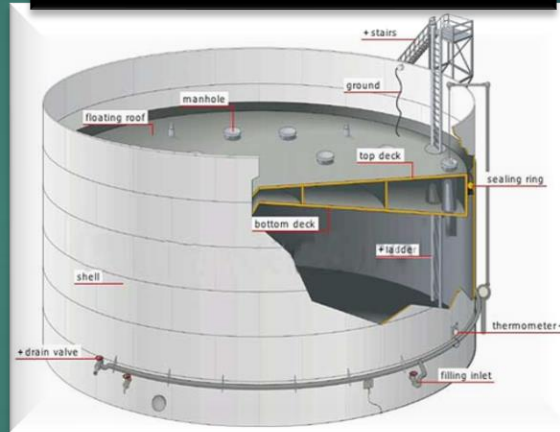
External Floating Roof (EFR)
