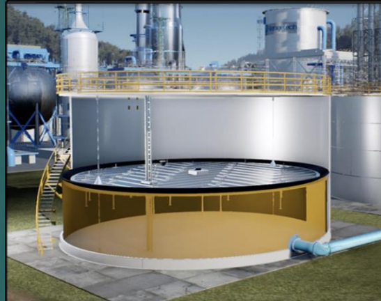
Internal Floating Roof (IFR)
