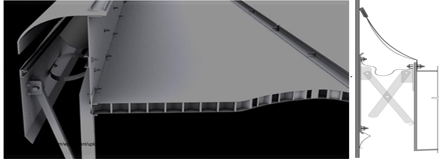
Primary Seal “Mechanical Shoe” with a Secondary wiper seal
