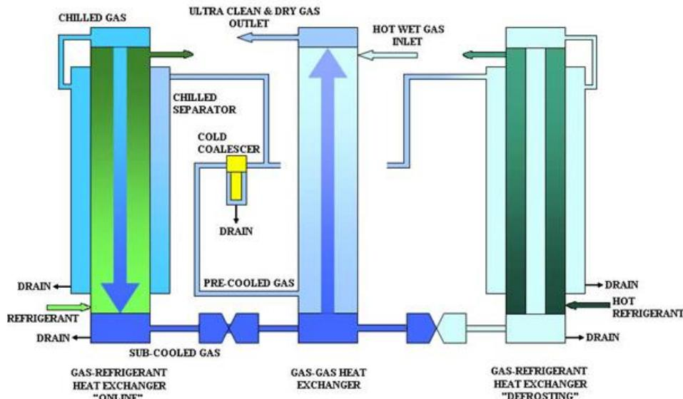
Figure 3. Pioneer Total Contaminant Removal (TCR) System
