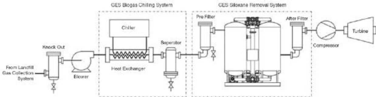
Figure 8. Typical Parker GES Landfill Gas Flow Schematic
