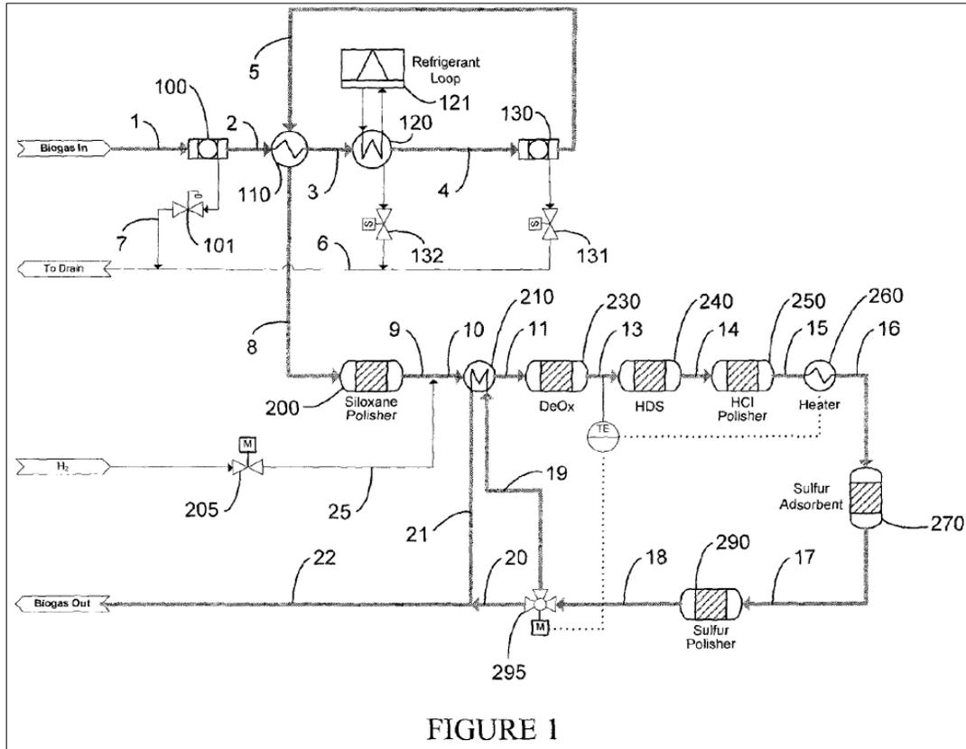
Figure 4. Quadrogen Biogas Cleanup System in Patent
