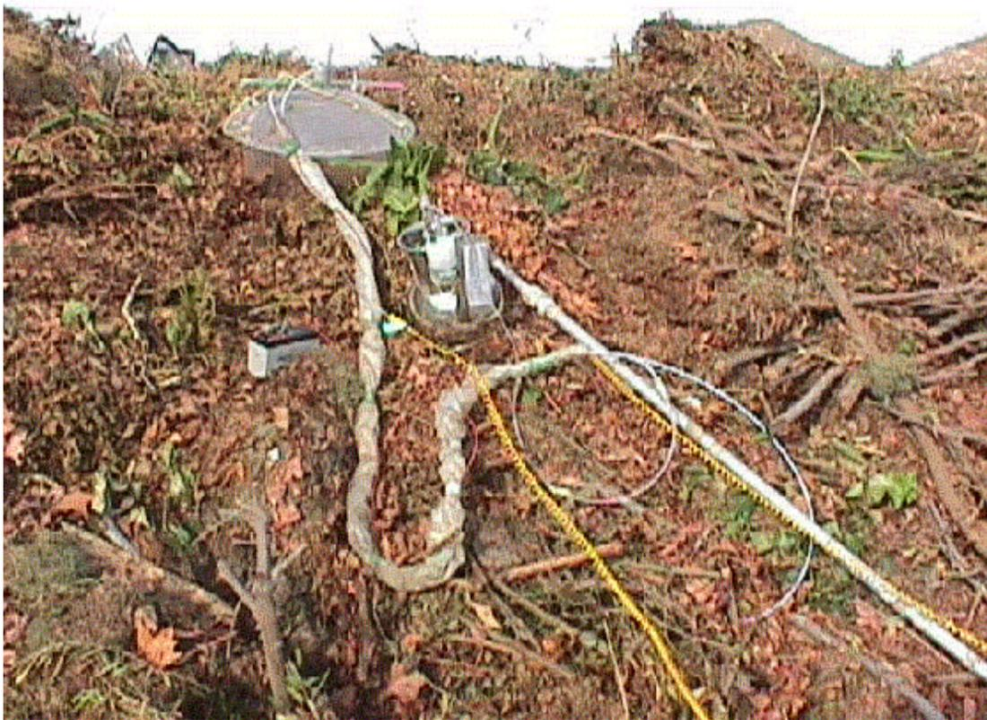
**Figure 6 – Photo of Tipping Pile and Flux Chamber**
