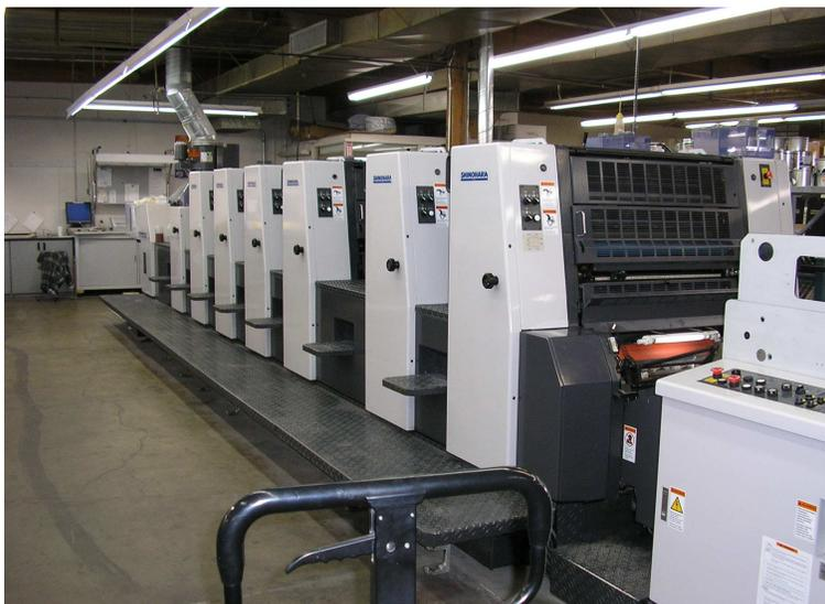
Figure 2-14. Six Color Press at The Printery
