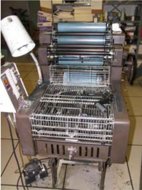
Figure 1-2. Rollers on Small Lithographic Press
