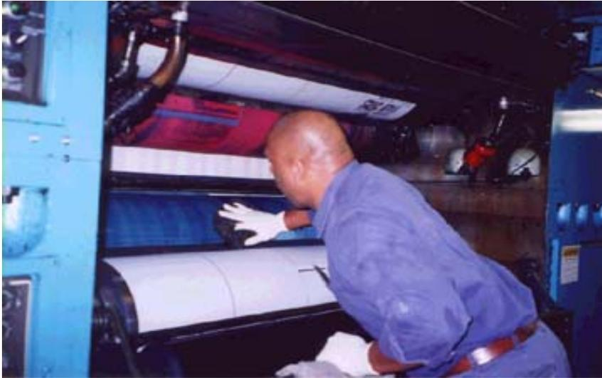
Figure 1-1. Blanket on lithographic printing press
