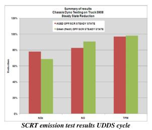
The system also demonstrated 68-78% NO<sub>x</sub> reduction during a 30 mph steady state test.
