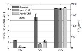
Figure 5. Regulated emissions comparison from different exhaust configurations over the UDDS cycle.
