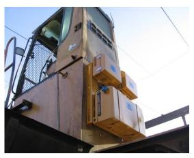
Figure 2. DPF/SCR Components on Excavator
