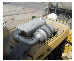
Figure 1. DPF and SCR Catalyst on Loader
