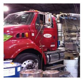
Figure 1. Test Vehicle during chassis dynamometer testing.
