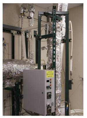
Figure 1. Picture of SHR-WGS systems. SHR (left) was modified and new WGS (right) was added.
