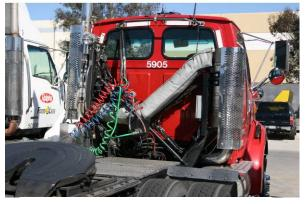
Figure 15: Truck Equipped with SCRT<sup>TM</sup>
