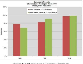
Figure 16: Chassis Dyno Testing Results on Truck 5908 Steady State Reduction
