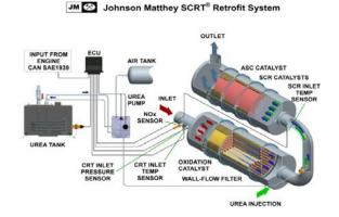
The CRT was previously verified by ARB as a level 3 PM control device (>85% reduction) that also meets the 20% NO2 requirement for 1998-2002 MY heavy duty diesel engines. The SCR system uses NH3, carried on the vehicle as urea, to reduce  $NO_x$  over a vanadium based catalyst. The precise air assisted injection of urea is performed using an OE dosing pump controlled by an ECU that was developed by JM.
