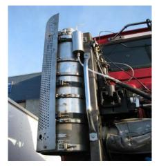
Figure 2. SCRT system installed on the test vehicle.
