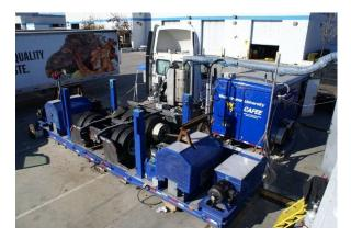
Figure 5: WVU Transportable Chassis Dynamometer
