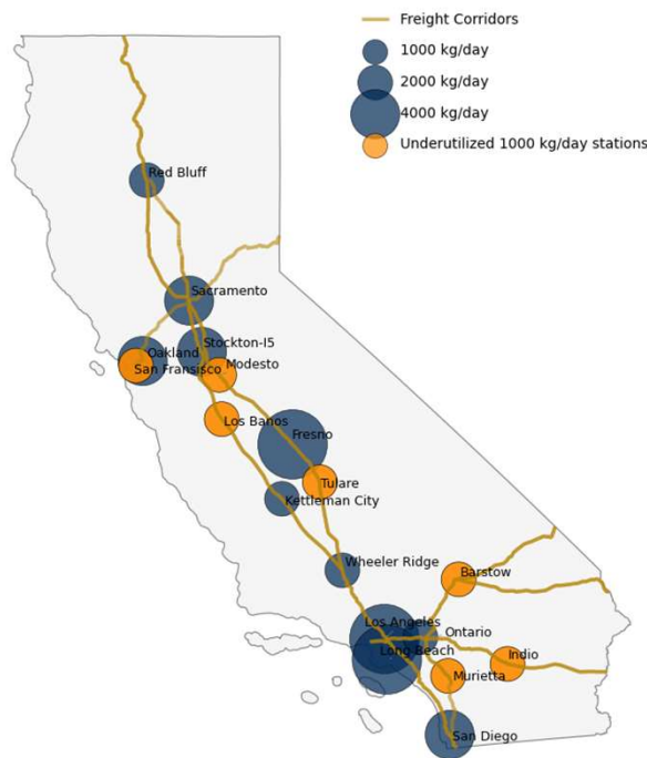
Hydrogen Refueling Station Siting: 1000 Trucks
